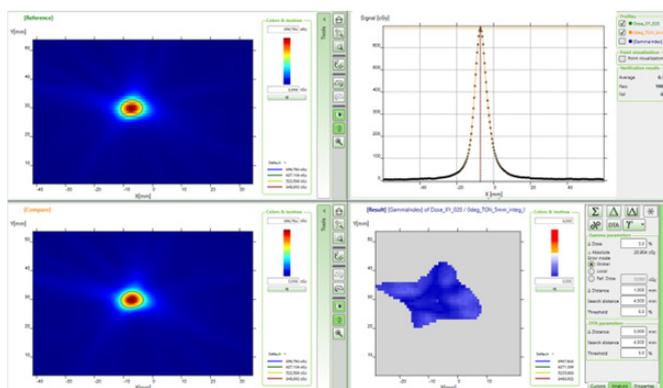
Figure 2. Pre-treatment validation of the CyberKnife® plan with a small 5 mm target. Top left—TPS calculated dose, bottom left—myQA® SRS measured dose; top right— profile through the target volume center with representation of the measurement points; bottom right—gamma analysis at 3%/1mm with a 100% passing rate.
