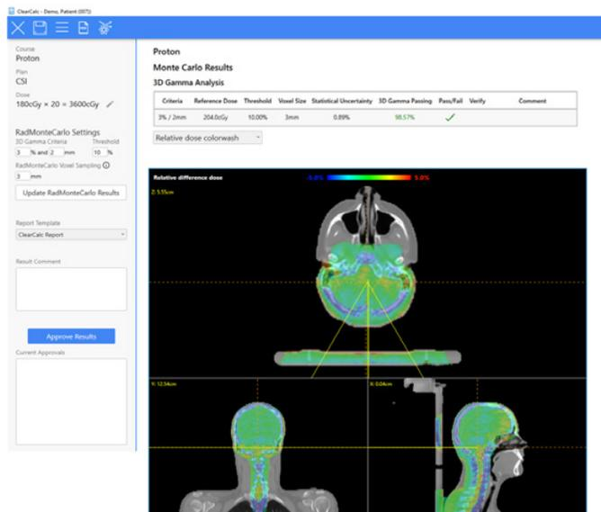
Figure 2. Secondary calculations in ClearCalc showing RadMonteCarlo volumetric 3D gamma analysis for a CNS proton plan.
