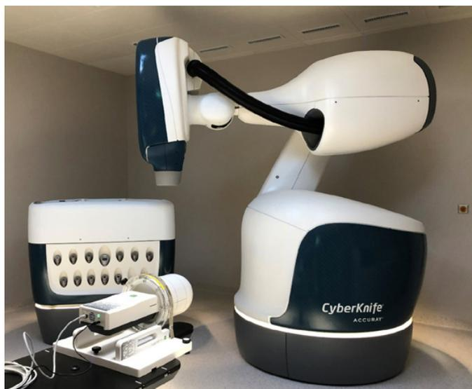
Figure 1. myQA® SRS used for CyberKnife® QA
