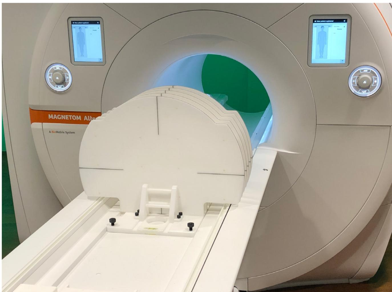
Figure 2. Enhanced imaging, enhanced outcome: the THETIS 3D MR Distortion Phantom enables streamlined QA workflows for the safe deployment of MRI systems in a radiotherapy setting.
