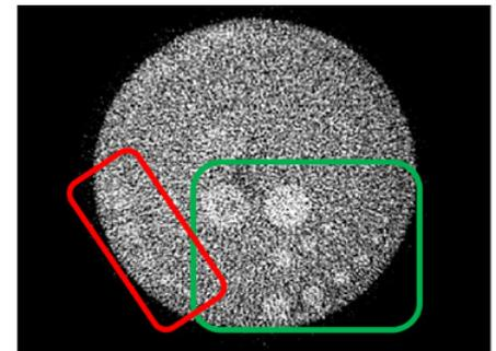
Figure 2. Low Contrast Detectability of a CBCT scan on IQphan. The higher contrast and larger diameter objects are critical for achieving useful measurements.
