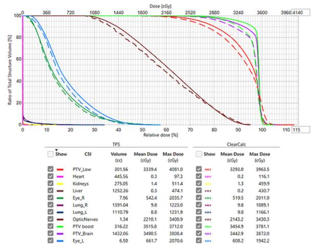
Figure 3. 3D dose volume histogram and dose constraint information for a proton plan with ClearCalc and RadMonteCarlo.
