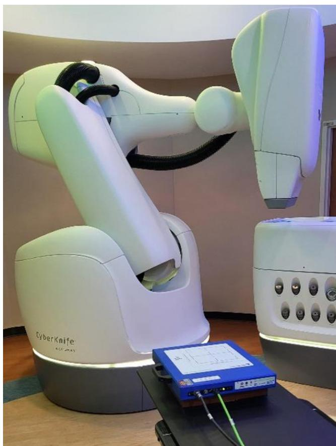
Figure 1. QA StereoChecker set up on CyberKnife couch.
