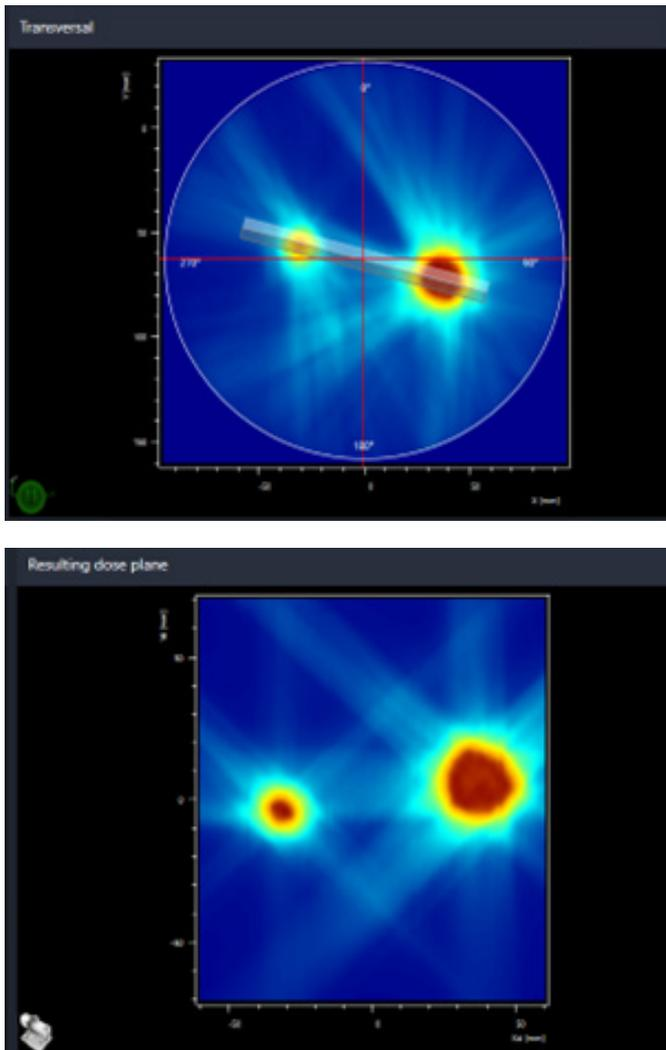
Figure 3. myQA® Plane Viewer Tool— with the detector rotation of ~15 degrees (left), one is able to QA high dose regions of both target volumes at the same time (right).
