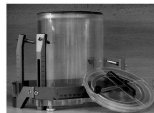
Fig. 1. The inhouse made cylindrical Perspex phantom secured to the base of the Leksell stereotactic frame was used for measurements made in this study.
